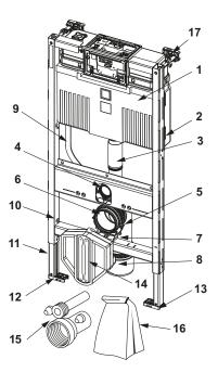
9300380 – TECEprofil toilet module with Uni cistern for universal connection of a shower toilet, installation height  $820 \, \text{mm}$
