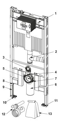
$9300502-TECE profil \ to ilet\ module\ with\ Octa\ II\ cistern,\ 8\ cm,\ installation\ height\ 1120\ mm$
