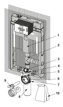
$9370032-\mbox{TECEbox}$  washstand module, installation depth 8 cm
