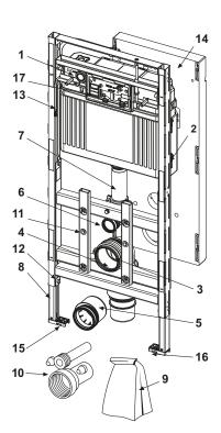
9600400 – TECElux toilet module 400, subsequent height adjustment, with odour extraction, installation height 1120 mm
