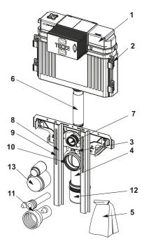
9510003 - TECE washstand support for the installation in metal or wooden stud walls
