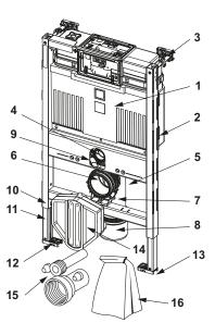
9300102 – TECEprofil toilet module with Uni cistern, with integrated warm and cold water hygiene flushing function, installation height 1120 mm
