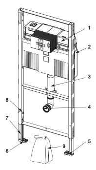
$9300382-{\mbox{TECEprofil}}$  toilet module with Uni cistern for universal connection of a shower toilet, installation height  $980\mbox{ mm}$
