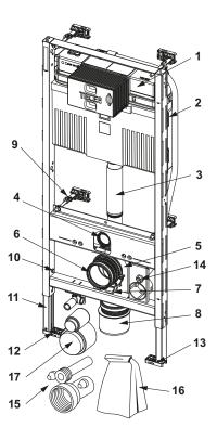
9300309 – TECEprofil WC Geronto module with Uni cistern, ceramic attachment for sitting height of 48 cm in keeping with German standard DIN 18040-1, installation height 1120 mm
