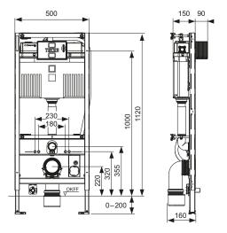
TECEprofil WC Geronto module with Uni cistern, ceramic attachment for sitting height of 48 cm in keeping with German standard DIN 18040-1, installation height 1120 mm
