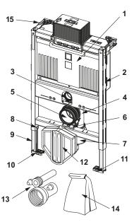
9300344 – TECEprofil toilet module TECEprofil with Uni cistern, for TOTO Neorest Washlet (WC) AC 2.0/EW 2.0, installation height 1120 mm
