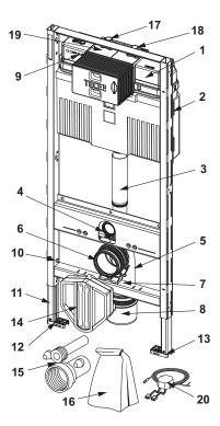
$9300103- TECE profil to ilet \ module \ with \ Uni \ cistern, \ with \ integrated \ cold \ water \ hygiene \ flushing function, installation height \ 1120 \ mm$
